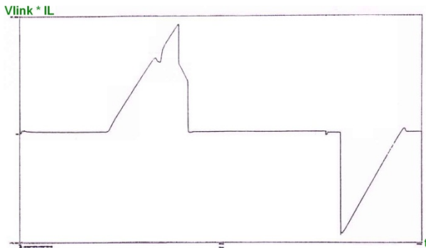
Fig. 9. Wasted energy in the proposed resonant link (Vlink(t) * IL(t))
