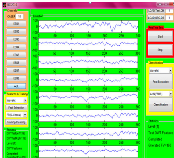
Fig. 5. The GUI of the proposed EEG- based non-invasive BCI system.
