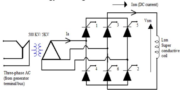
Fig. 3. SMES unit with six-pulse bridge ac/dc thyristor controlled converter
