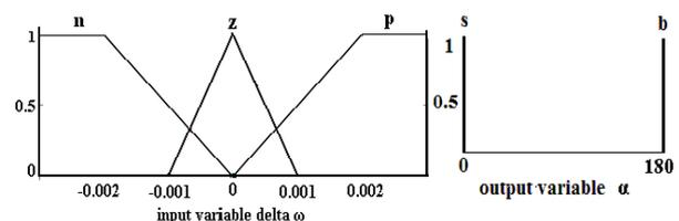
Fig. 5. Membership functions of input variable  $\Delta\omega$ (pu) and output variable  $\alpha$  for Braking Resistors.
