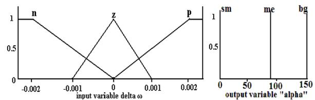
Fig. 4. Membership functions of input variable  $\Delta\omega$ (pu) and output variable  $\alpha$  for SMES
