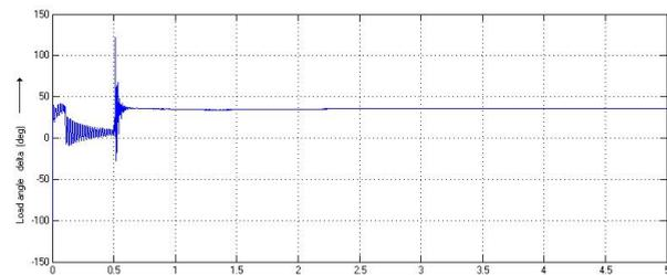
Fig. 8. Load angle response with power system stabilizer under 3LG fault
