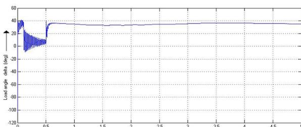
**Fig. 11.** Load angle response with fuzzy controlled SMES under 3LG fault
