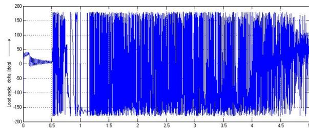
Fig. 7. Load angle response without power system stabilizer under 3LG fault
