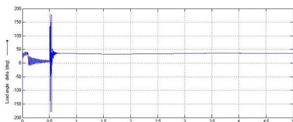
**Fig. 10.** Load angle response with fuzzy controlled Braking Resistor under 3LG fault
