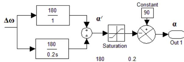
Fig. 6. Block diagram of PI controller
