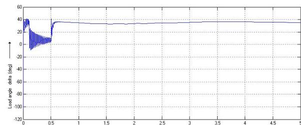
Fig. 9. Load angle response with PI controlled SMES under 3LG fault
