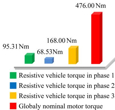
**Fig.11.** Evaluation of the globally vehicle resistive torque compared to nominal motor torque in different phases
