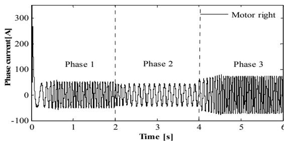
Fig. 9. Variation of phase current of the right motor in different phases.
