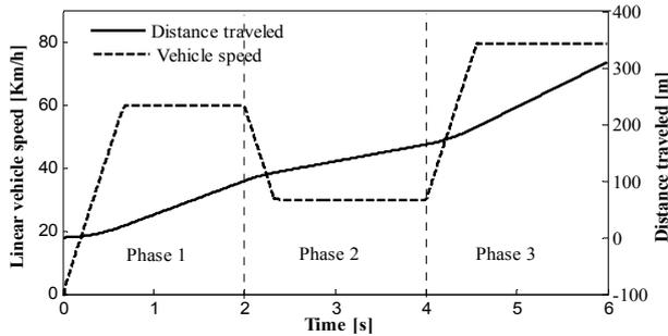
Fig. 8. Evaluation of vehicle and distance travelled in different phases
