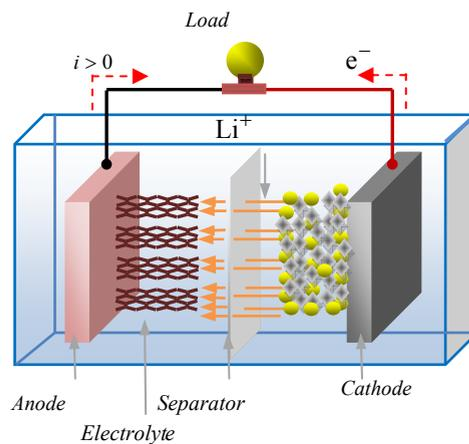
Fig. 3. Lithium-ion battery charge diagram.
