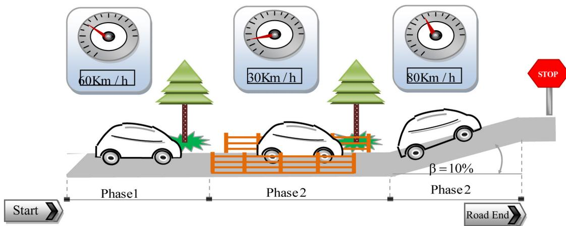
Fig.6. Specific driving road topologies
