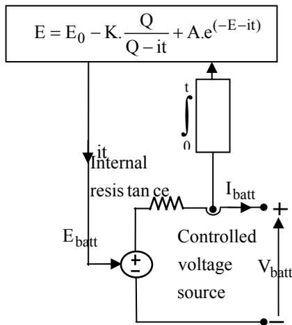
Fig. 4. The equivalent circuit of Lithium-ion battery.
