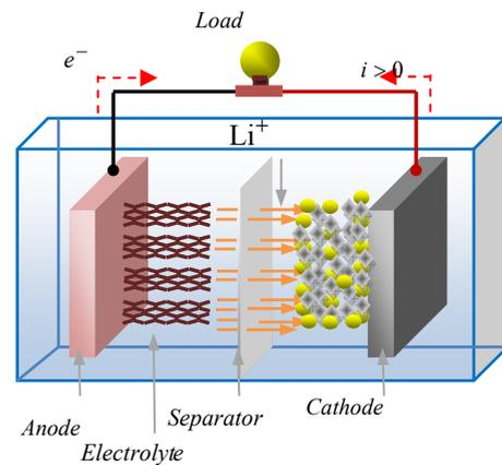
Fig. 2. Lithium-ion battery discharge diagram.
