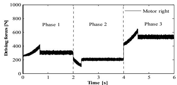
Fig. 10. Variation of driving force of the right motor in different phases
