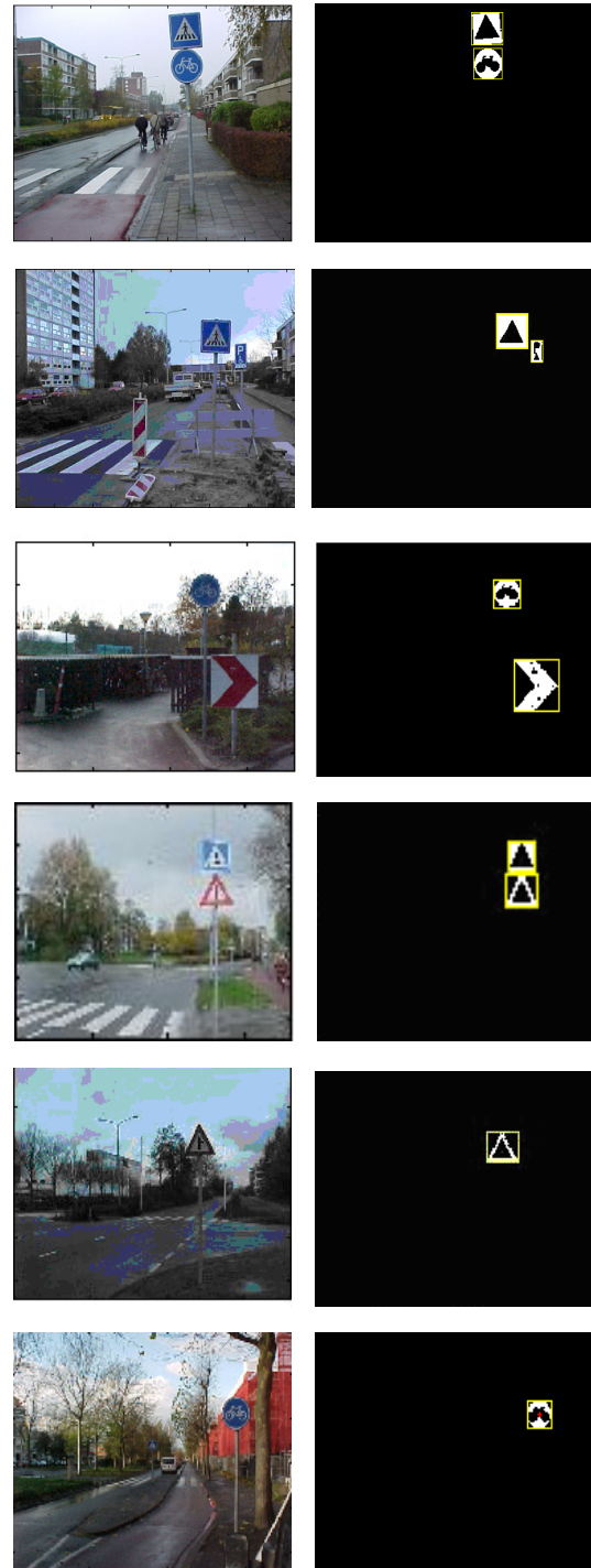
Fig. 7. Detection and segmentation of road signs in natural scene, input image (first column), and segmented sign (second column).
