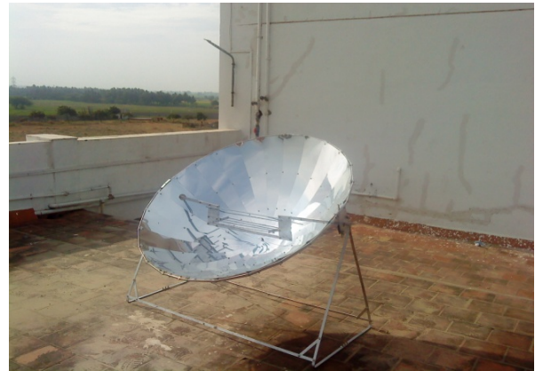
Fig. 1. Parabolic Collector with Aluminium Reflector
