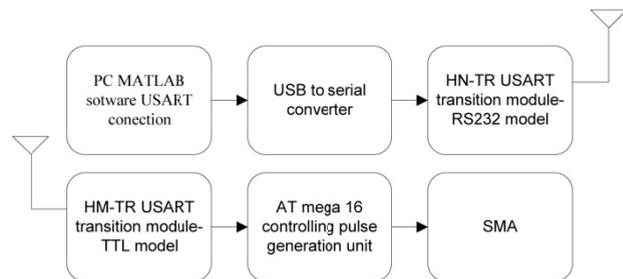
**Fig. 15.** The block diagram of robot control
