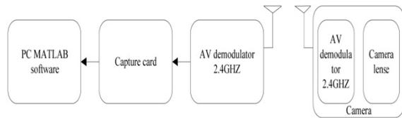
Fig. 16. Block diagram of the robot imaging
