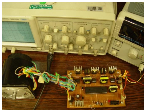
Fig. 13. The purposed sensor-less controller test system
