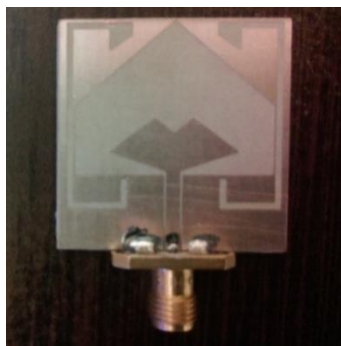
Fig. 13. Photograph of the fabricated UWB microstrip antenna.
