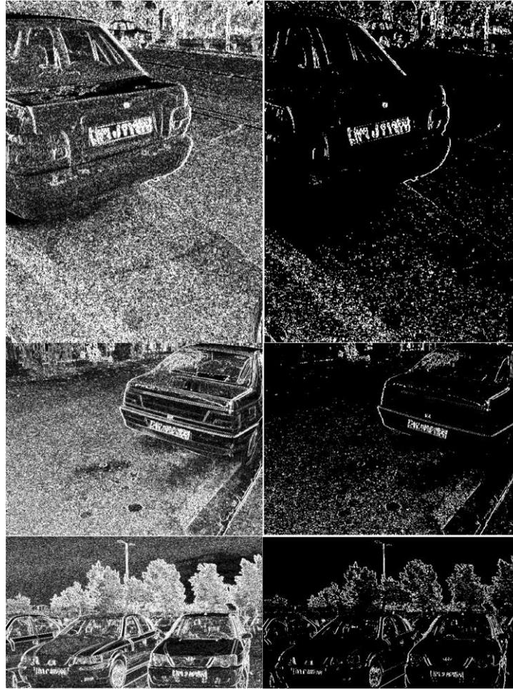
**Fig. 3.** The output of Sobel vertical edge detector without using a threshold (left-column) and with using the threshold value based on (11) (right-column).
