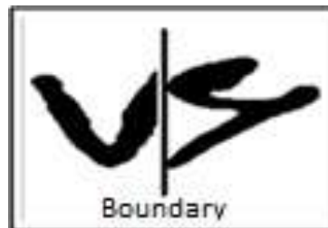
Fig. 3. Segmentation of the image into two isolated digits using concatenated HMM.
