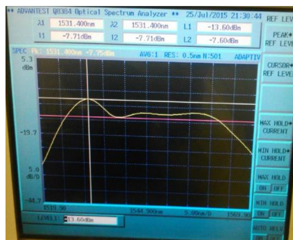
Fig. 2. The simulation and experimental output spectrum of backward ASE
