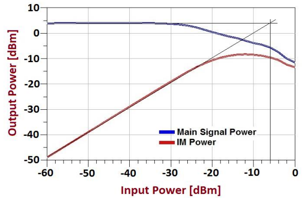
Fig. 6. IIP3 with two input RF signals of 5.0 GHz with 100 MHz frequency spacing
