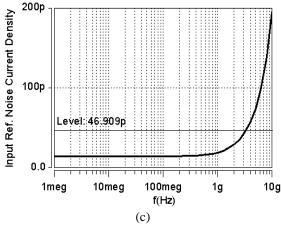
**Fig. 12**. (a) Output noise (b) Input referred noise of the proposed TIA. (c) Input referred noise of the TIA without feedback system.
