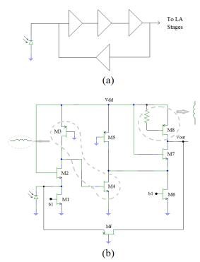
Fig.2. a) Block diagram.0m b) Proposed TIA circuit
