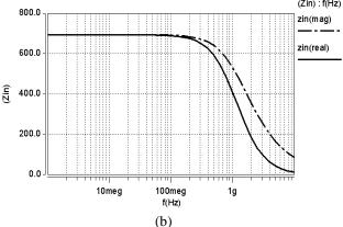
**Fig. 5.** Input impedance and input resistance (a) with feedback (b) without feedback network.
