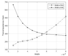
Fig. 10. Width of M5 and M4 vs. gain
