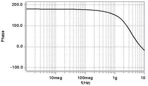
**Fig. 4.** (a) Frequency response (b) Phase of the proposed TIA.
