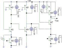
Fig. 11. Equivalent noise circuit
