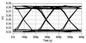
Fig. 6. Simulated Eye-Diagram of the Proposed TIA for 100µA 5Gbps NRZ PRBS7
