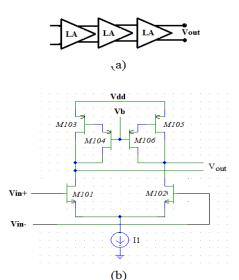
**Fig. 13.** (a) Block diagram of the Limiting Amplifier (b) Structure of each cell gain
