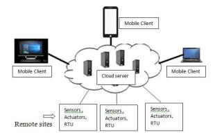
Fig. 7. The general architecture of SCADA systems in an IoT-cloud environment [11].
