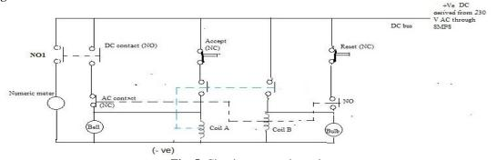
Fig. 5. Circuit on control panel.
