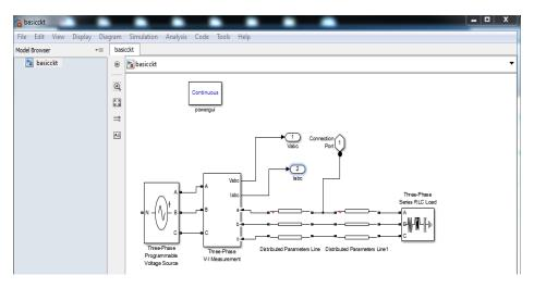
Fig. 1. Modeling of Transmission Lines.
