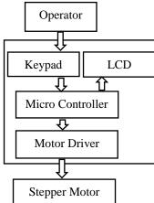
Fig. 5. The block diagram of the controller.
