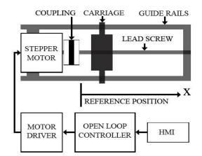
Fig. 4. The schematic model of the mechatronic part.
