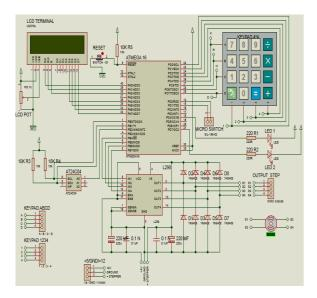
Fig. 6. The designed controller unit.
