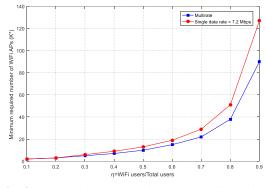
Fig. 8. The minimum required number of APs in two modes of single-rate and multi-rate WiFi AP with Nov=200.
