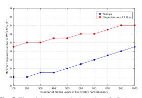
Fig. 5. The minimum required number of APs in two modes of single-rate and multi-rate WiFi AP with  $\eta$ =0.7.
