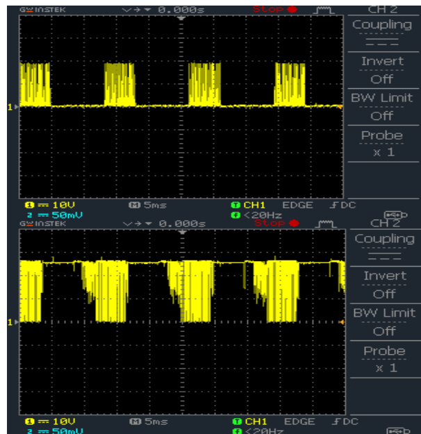
Fig. 19. Waveforms between MOSFET circuits and phases A and B.
