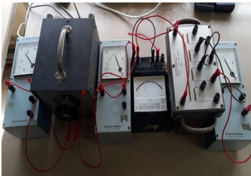
Fig. 8. Practical connection of transformer short-circuit test.
