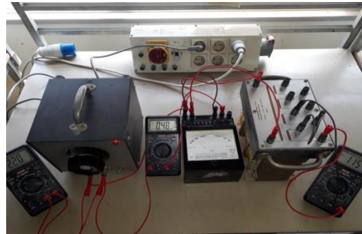
Fig. 6. Practical connection of transformer open-circuit test.
