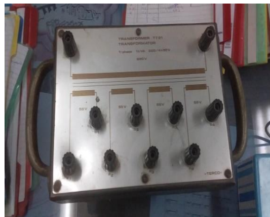
Fig. 1. Real 1KVA transformer (Terco-type).
