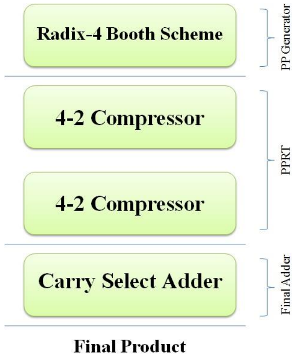
Fig. 5. Proposed concept for implementation of 16×16 bit Booth multiplier.
