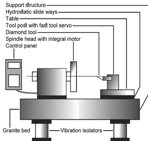
**Fig. 1.** A typical single-point diamond turning machine components [1].
