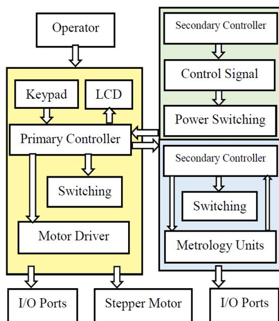
**Fig. 2.** Schematic diagram of the developed MAAHC [42].
