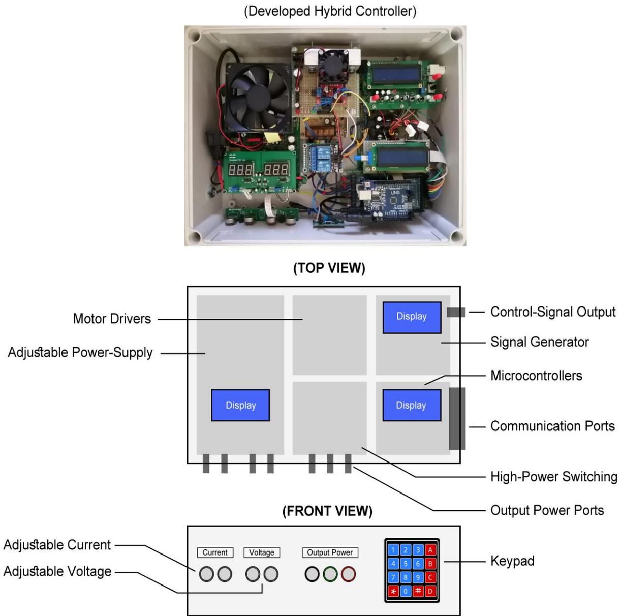
**Fig. 3.** The developed MAAHC and schematic views of the device.
