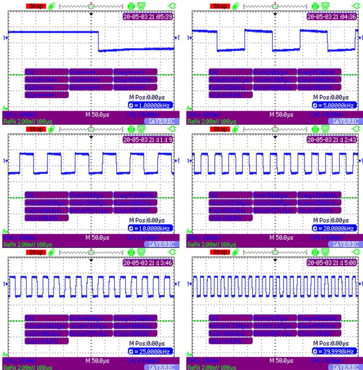
**Fig. 5.** The generated control signals for driving the active vibration systems: 1 KHz, 5 KHz, 10 KHz, 20 KHz, (D) 25 KHz, and 40 KHz.
