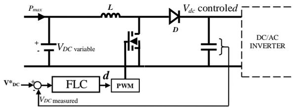
Fig.10. FLC regulation of DC-DC BOOST voltage Regulator.
