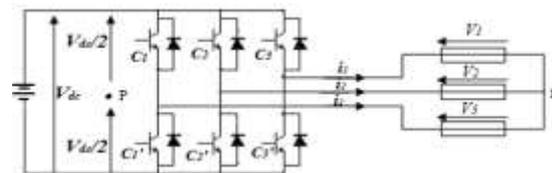
Fig. 8. Electrical structure of a three-phase inverter with two levels.
