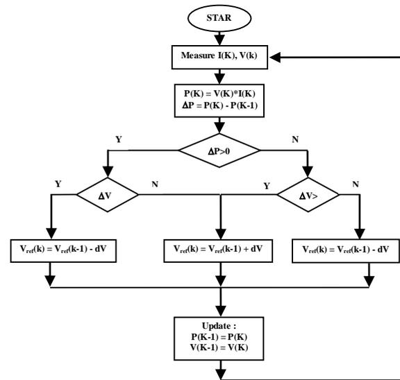
Fig.12. MPPT Algorithm by P&O
