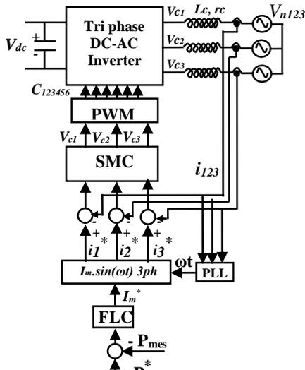
Fig. 11. SMC regulation in cascade with the FLC regulation of DC/AC Inverter.
