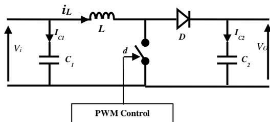
Fig.7. Structure of a DC/DC Boost Converter
