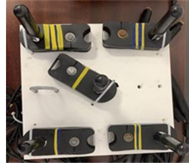
Fig. 2. The hydrophone array.
