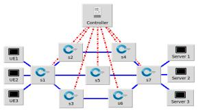
Fig. 3. The topology of the SDN-based scenario.
