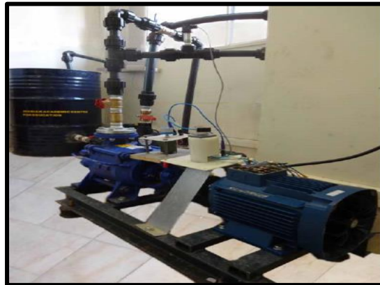
Fig. 2. Electro-pump system in system identification Lab., Iran Univ. of Sci. & tech.
