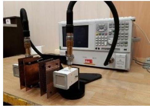
Fig. 3. The setup for measuring the reflection coefficient and coupling of two quad-ridge antennas in the presence of the EBG metasurface.
