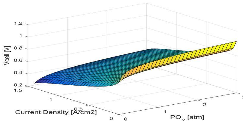
**Fig. 3.** Variation of PEMFC cell voltage as a function of current density and oxygen pressure with ( $P_{H_2}=P_{H_2O}=1$  (atm),  $RH=100\%$  and  $T=90^\circ C$ ).
