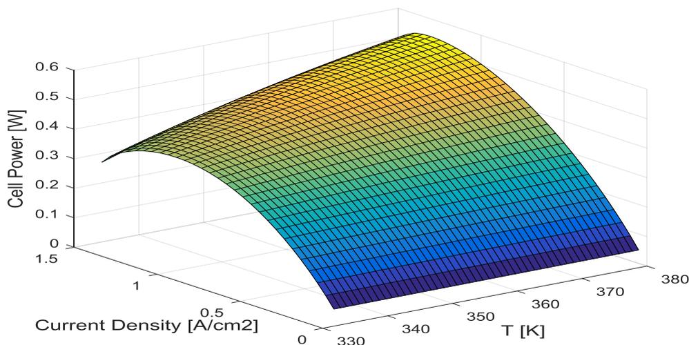
Fig. 7. Changes in cell power as a function of current density and temperature over time ( $P_{H_2}=P_{O_2}=1(atm)$  and  $RH=100\%$  ).
