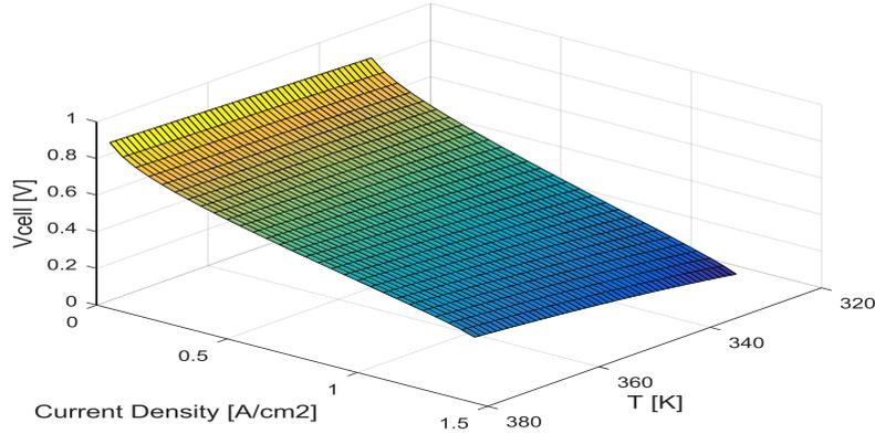
**Fig. 8.** Cell voltage variation as a function of current density and temperature with ( $P_{H_2}= P_{O_2}= 1(atm)$  and  $RH=100\%$  ).
