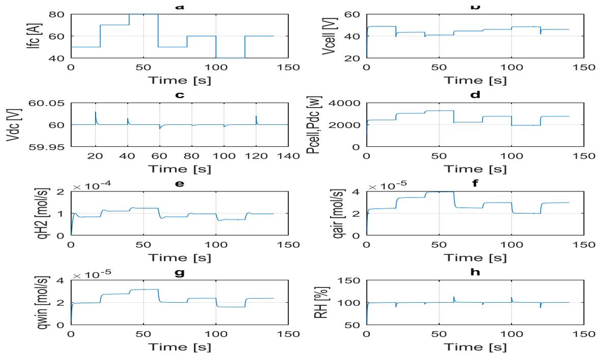
Fig. 11. PEMFC operational variables are under control.
