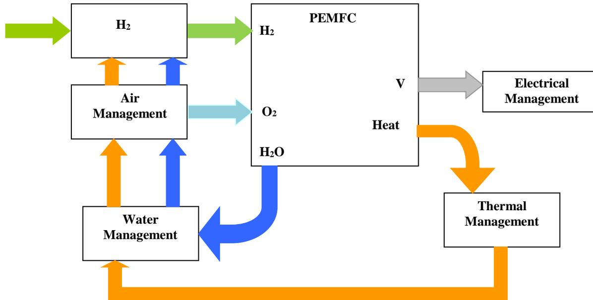
Fig. 1. Synoptic diagram for an operating fuel cell model [3]-[23].
