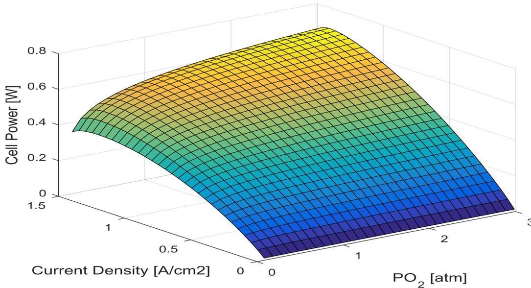
**Fig. 4.** Variation of PEMFC cell Power as a Function of Current Density and Oxygen Pressure with ( $P_{H_2}=P_{H_2O}=1(atm),RH=100\%$  and  $T=90^\circ C$ ).
