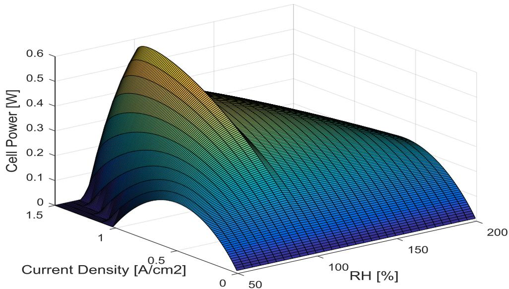
**Fig. 5.** Changes in cell power as a function of current density and relative humidity over time ( $P_{H_2}=P_{O_2}=1(atm)$  and  $T=90^\circ C$ ).
