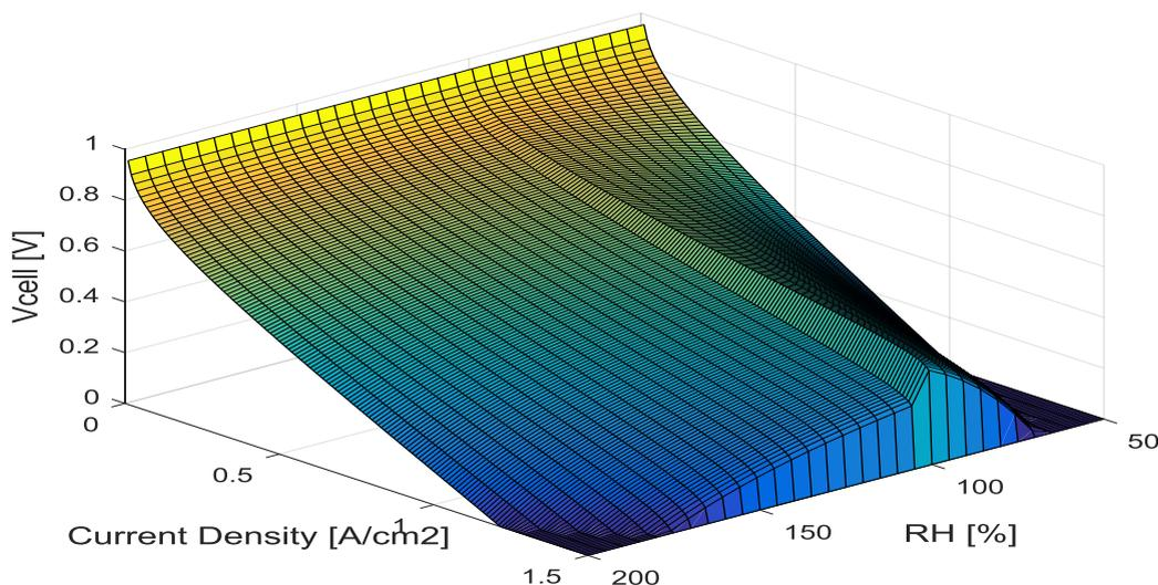
Fig. 6. Variation of cell voltage with respect to current density and relative humidity ( $P_{H_2}=P_{O_2}=1(atm)$  and  $T=90^{\circ}C$ ).
