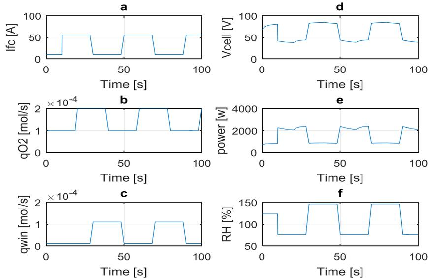
**Fig. 9.** The dynamic characteristics of a PEMFC (*I<sub>fc</sub>*, *q<sub>O2</sub>*, *q<sub>H<sub>2</sub>Oin</sub>*, *V<sub>cell</sub>*, *P<sub>cell</sub>* and *RH*).
