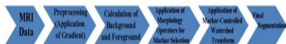
Fig. 15. The block diagram of the proposed marker-controlled watershed transform algorithm for brain MRI segmentation
