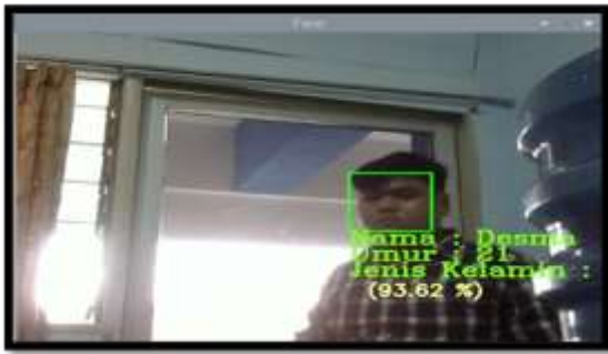
Fig. 5. Implementation of the Local Binary Pattern Histogram Algorithm.
