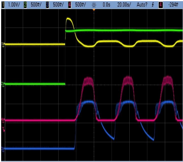
Fig. 14. Hardware Results: Battery Current, Battery Voltage, PV Voltage & PV Current.
