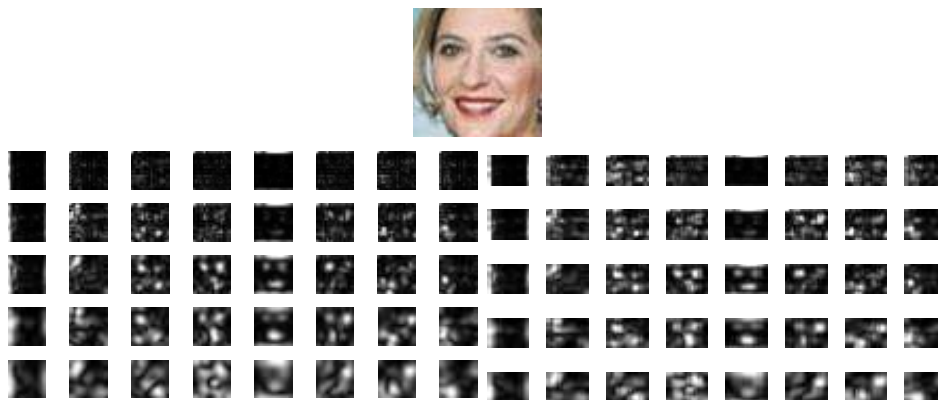
Fig. 3. Output of each stage of scattering wavelet transform in one scale and eight directions.
