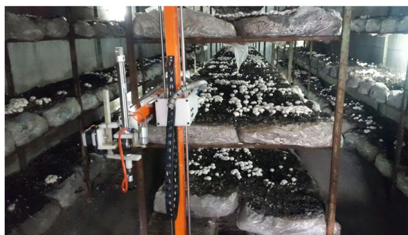
Fig. 3. Mushroom harvesting robot while working on the substrate.
