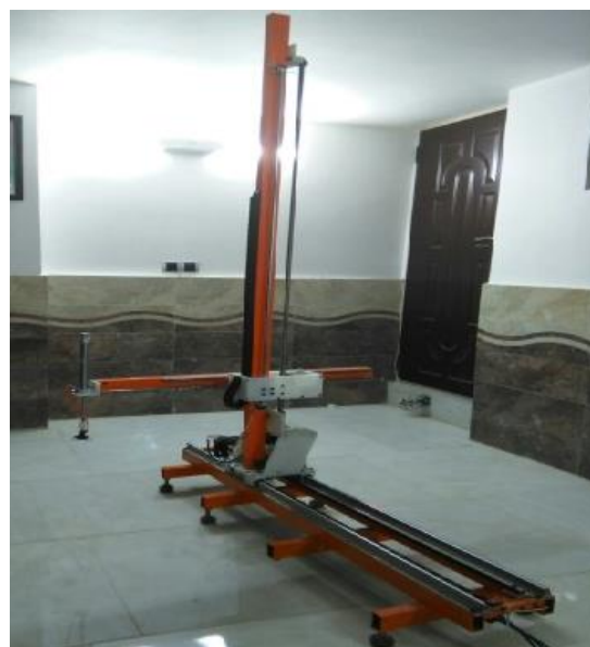
Fig. 2. Developed mushroom harvesting robot in the current research.
