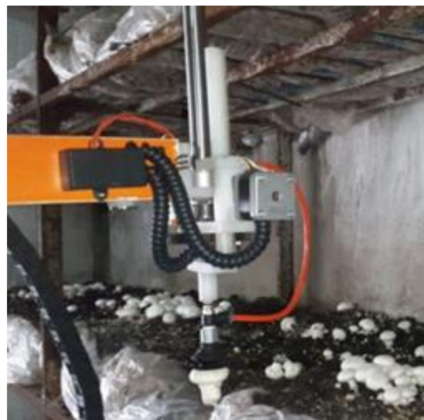
Fig. 4. End-effector during harvesting.
