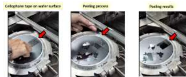
Fig. 12. Wafer surface peeling test procedure.
