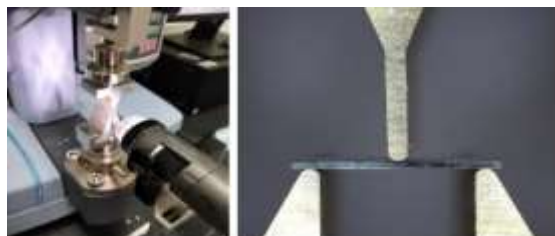
Fig. 17. Camera feature to ensure consistent die positioning on jig during three-point bending test.
