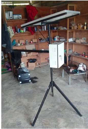
Fig. 4. Real Design of flood detection tool using HC-SR04 sensor based on Virtuino.
