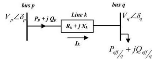
Figure 1. The model of two buses in a system.
