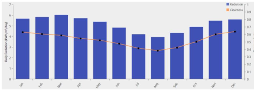
Figure 3. Average monthly solar radiation and clearness index of the study location.
