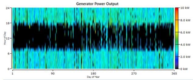
Figure 7. Diesel generator operating pattern proportionate fuel consumption.
