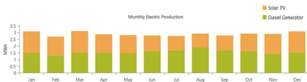
Figure 6. Average monthly electricity production of the hybrid system.
