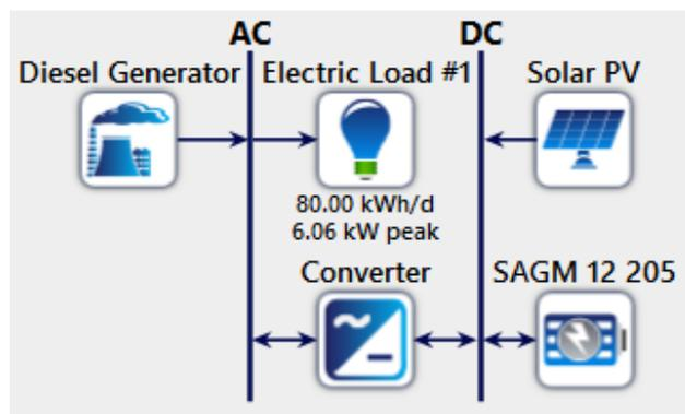
Figure 4. Schematic of the system setup.
