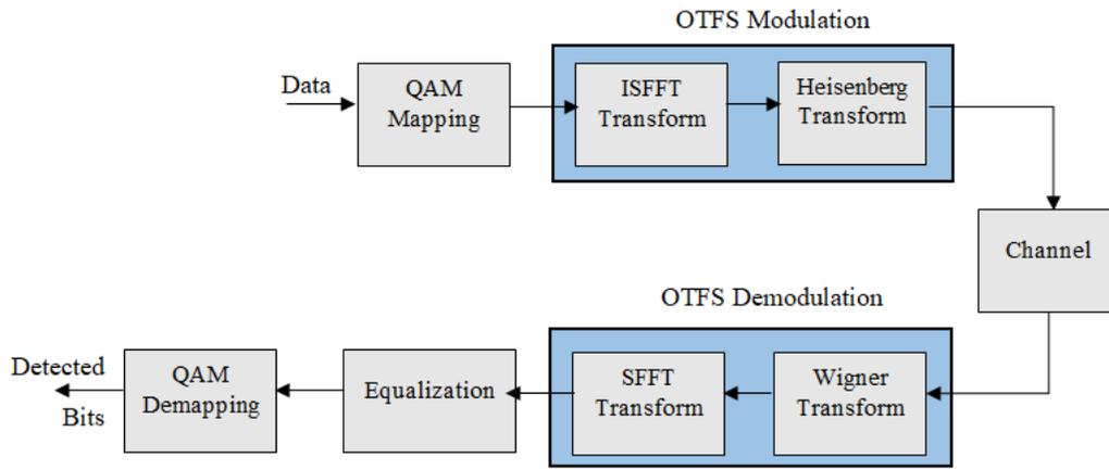
Figure 1. OTFS-based communication system.
