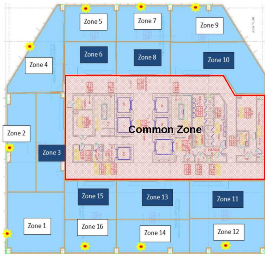
**Figure 4.** Lighting zoning plan with photocell and motion sensors for energy-efficient lighting control.
