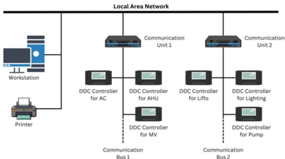
Figure 9. The network configuration of the EMS.
