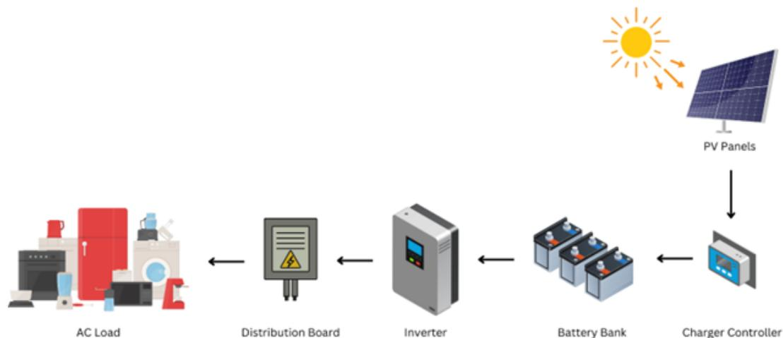
**Figure 6.** Proposed solar PV system configuration for GBI compliance.
