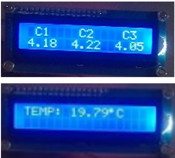
Figure 5. BMS data were displayed on an LCD screen.
