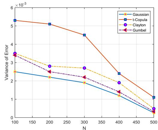
**Fig. 8.** Error variance of  $\sigma$  estimation using four types of copulas for  $S = 2$  and  $\sigma = 0.7$ .
