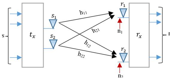
Fig. 1. A  $2 \times 2$  MIMO system model.
