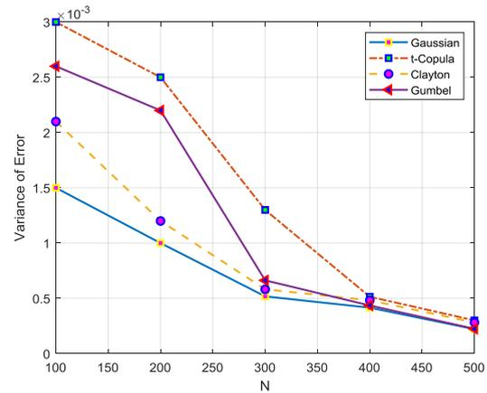
**Fig. 7.** Error variance of  $S$  estimation using four types of copulas for  $S = 2$  and  $\sigma = 0.7$ .
